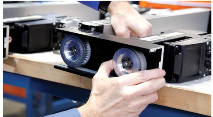
*Bosch Rexroth’s linear modules are very compact and feature high accuracy with repeatability in the five-micron range. The modules were combined to create a variety of kinematic solutions, such as Cartesian robot pick-and-place systems, incorporated into the DFP5000 cell.*
