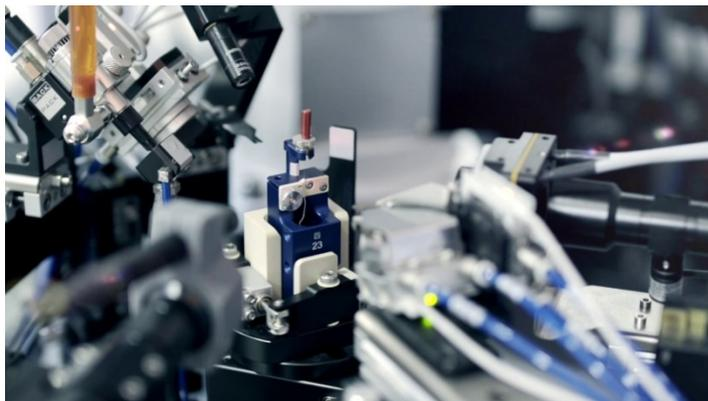
the trim station, a final adhesive dot is dispensed over the clipped wire stubs and UV cured. Inspection cameras then verify the adhesive on top of bead and the fibers below the bead.
