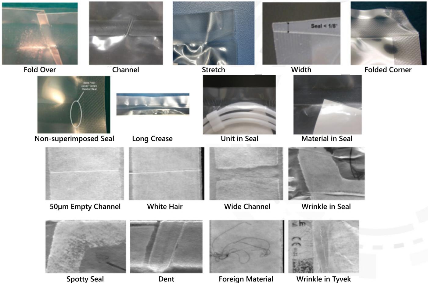
Figure 2 Understanding seal inspection requirements, including defect types, sizes, and packaging materials.
