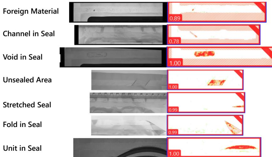
Figure 4. Package seal inspection results show the raw image (left) vs the processed images (right).
