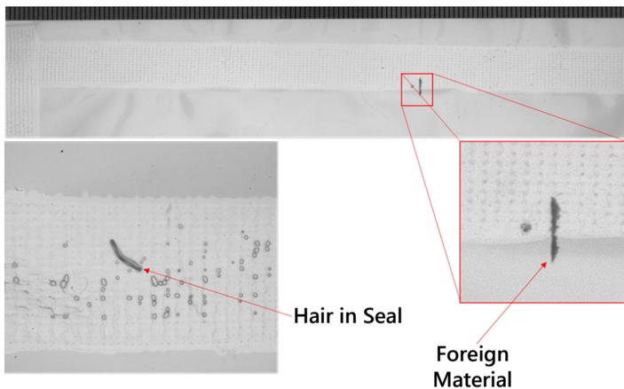
Figure 3. Area scan image of defects and voids in package seals.
