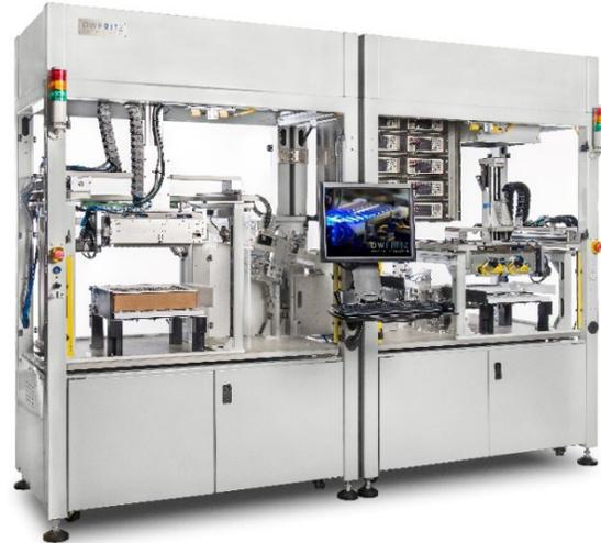
The ramp tilts, causing the cells to roll into a cell test station, where the system scans the bar codes of 10 cells and tests voltage and resistance against the manufacturer's test data with Kelvin probes and precision test instrumentation. Good cells are transported to the output module, where a second pick head places one row at a time into the battery module. Bad cells are diverted to a reject buffer.
